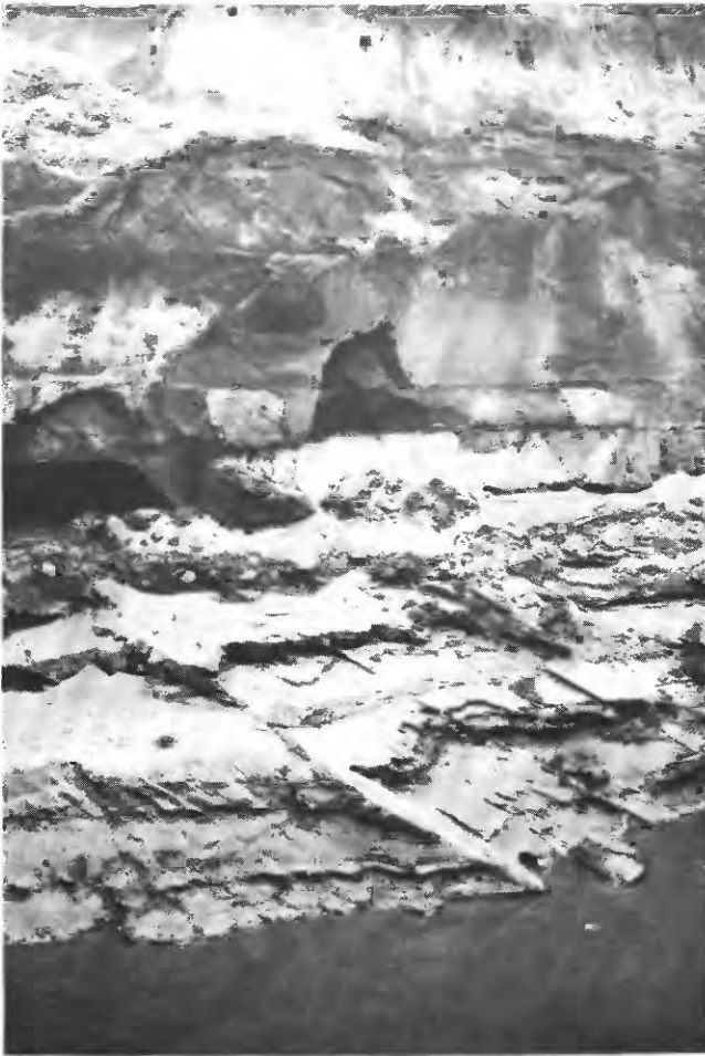
FIGURE 5.—Trail Ridge ilmenite ore sand exposed in 1984. The basal interval (about 0.9 m thick) is eolian sand with southwest-dipping crossbeds, overprinted by thin humate-cemented zones. Overlying lithologies are weakly cemented sand with crossbedding still visible (0.6 m thick), massive resistant humate-cemented sand (1.2 m thick), and at the top a rootlet-mottled bleached zone (the remainder). Location is shown on map in figure 7.
